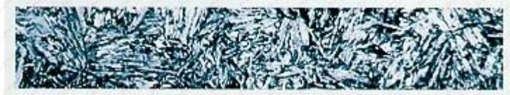
Too high hardening temperature gives coarse structure, high austenite content (30%), few carbides. Consequence: low hardness and bad wear resistance.
