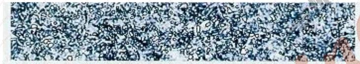
Optimized hardening conditions give optimal austenite content (15%), many uniformly distributed carbides.
