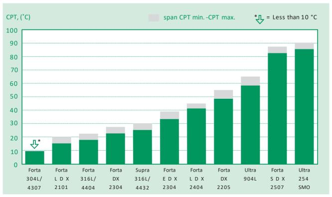
Typical critical pitting corrosion temperatures (CPT) in 1M NaCl measured according to ASTM G150 using the Avesta Cell. Test surfaces wet ground to 320 mesh. CPT varies with product form and surface finish.
