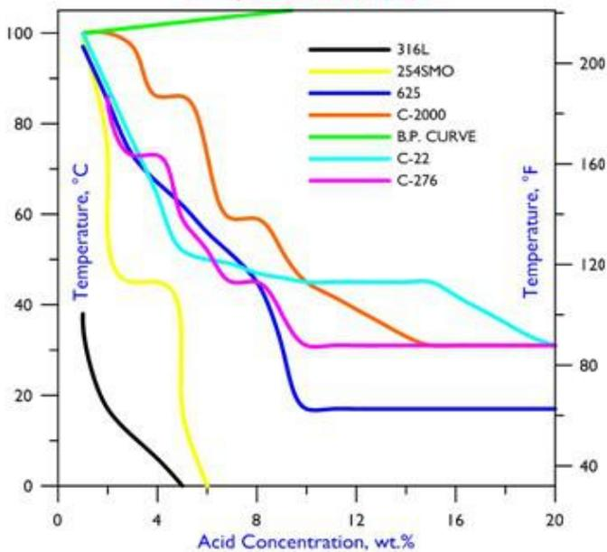
Comparison of 0.1 mm/y Lines in Sulfuric Acid
