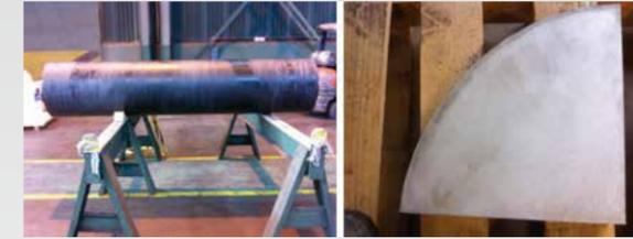
Figure 3 shows a Packer made out of alloy 945X intended for use in aggressive environment for an oil and gas well.
